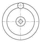
SAFETY SOLID HANDWHEELS VDN.FP+I+ST (see page 166) Duroplast
